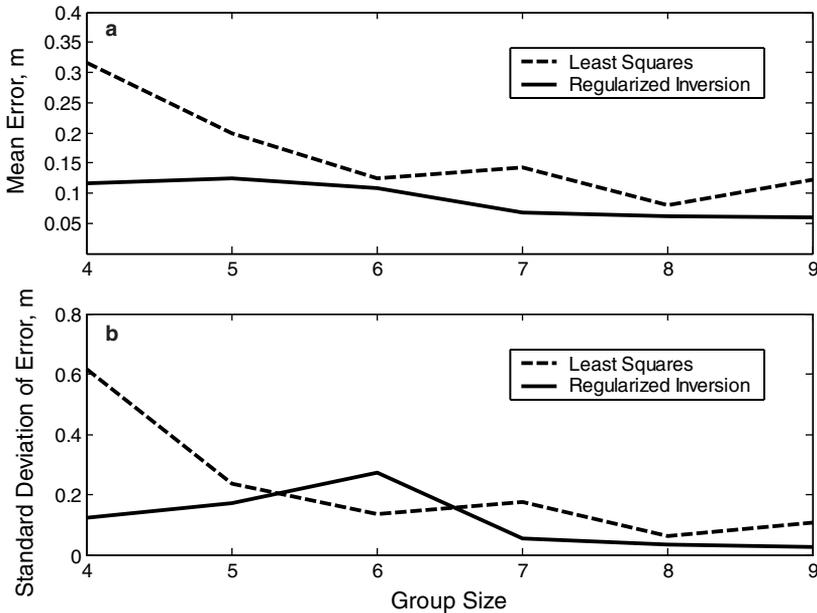
Fig. 2. The (a) average and (b) standard deviation of the RMS error in source position estimate as a function of group size. This includes all sources inside of the array area for the three arrays considered.
