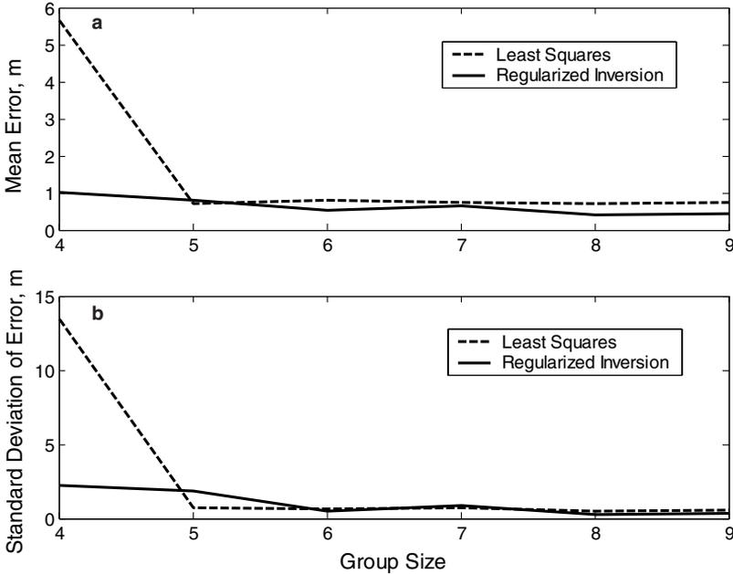
Fig. 5. The (a) average and (b) standard deviation of the RMS error in far-field source position estimate as a function of group size. This includes all sources outside of the array area for the three arrays considered.
