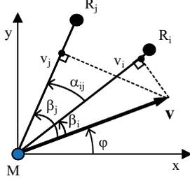
Fig. 3. Geometry of simplified setup for determining angular separation between two receivers.
