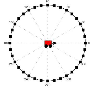
Fig. 5. Simulation setup. Anchor nodes are placed at  $1^\circ$  increments around the mobile node (some nodes not pictured for clarity).
