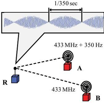
Fig. 1. Radio interferometry. Two nodes transmit sinusoidal signals at slightly different frequencies, which interfere to create a low frequency beat signal that can be measured by resource-constrained sensor nodes.
