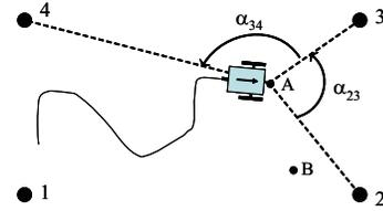
Fig. 2. A mobile sensor moves through the sensing region. The node navigates based on the angular separation between nodes (numbered 1 through 4).
